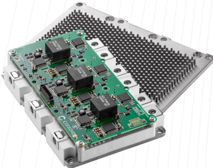
Our 3-phase 1200V Silicon Carbide (SiC) MOSFET Intelligent Power Module platform integrates high-performance power switches and gate drivers, built on the CISSOID HADES2® chipset. Designed for high power density applications, these modules enable efficient operation at junction temperatures up to 175°C, fully leveraging the benefits of SiC technology—namely, low switching losses and high thermal resilience.
