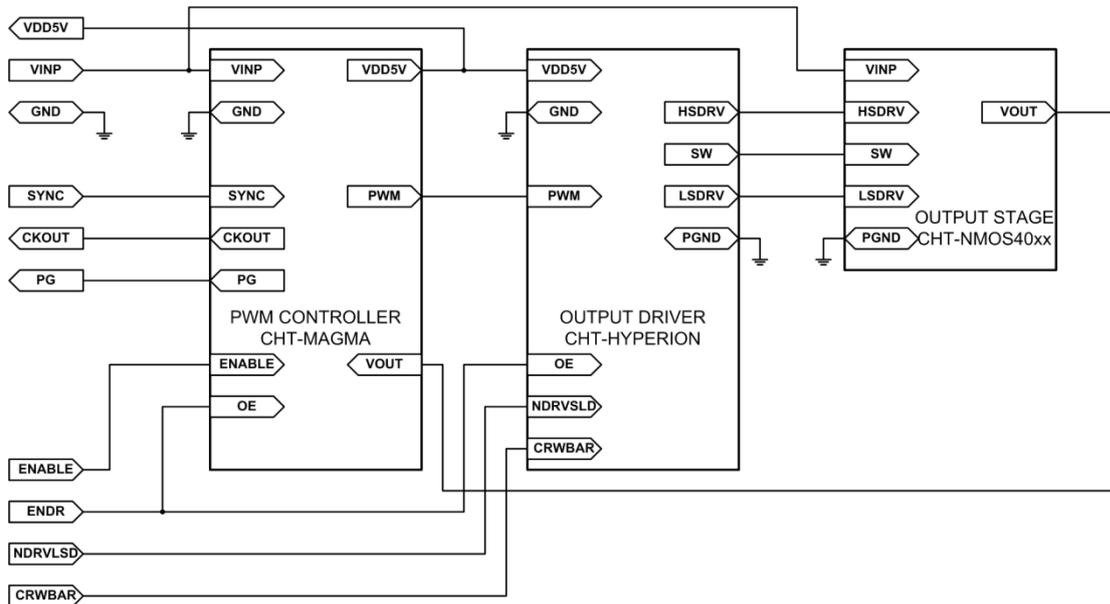
VESUVIO® DC-DC Converter Technology is based on a synchronous buck architecture which provides voltage step-down capability with high efficiency compared to traditional voltage regulator solutions.
