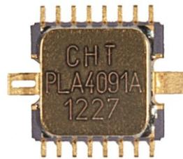
This transistor is capable of switching a current up to 1A (continuous) or blocking a voltage up to 80V with a drain cut-off current as low as 10uA at  $225^{\circ}\text{C}$ . In repetitive pulse conditions, it is able to handle peak currents up to 3.3A at  $225^{\circ}\text{C}$ .
