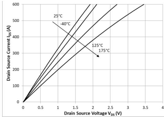
**Figure 1:** Drain current vs  $V_{DS}$  ( $V_{GS}=15V$ ,  $t_p < 200\mu s$ )<sup>11</sup>
