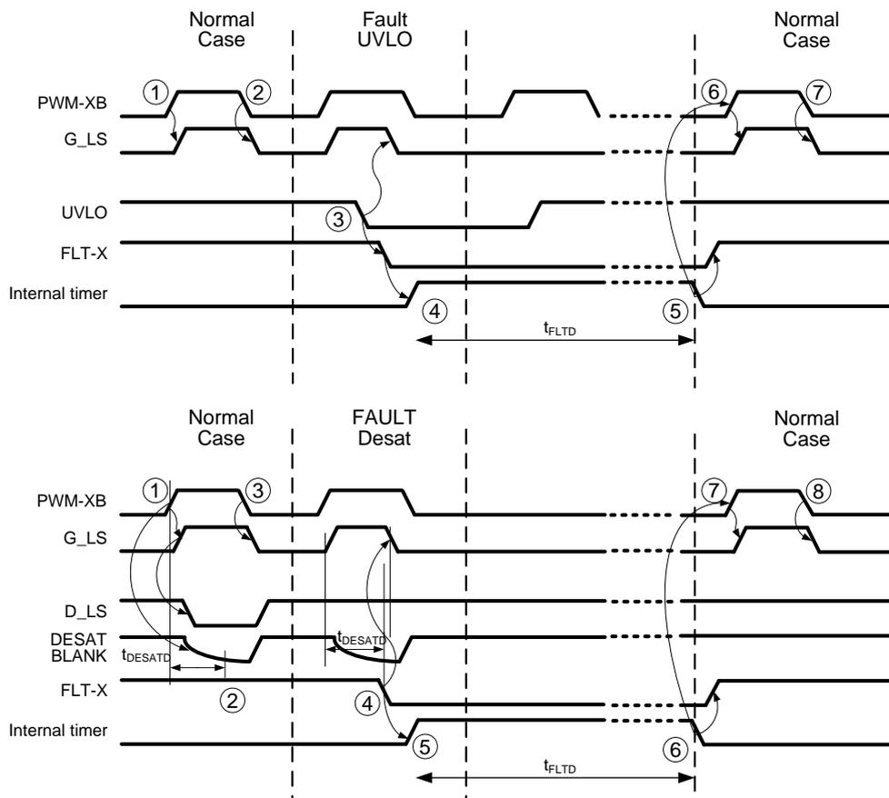
Figure 25: Timing diagram CXT-PLA3SA12450A low-side gate driver behaviour
