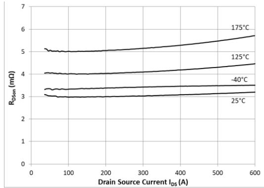
**Figure 2:** On-state drain source resistance vs. Drain current ( $V_{GS}=15V$ ,  $t_p < 200\mu s$ )<sup>11</sup>
