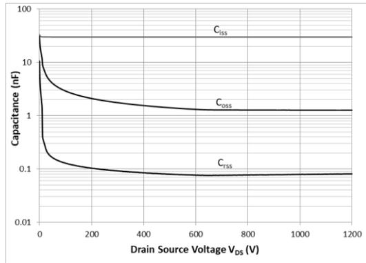
**Figure 8 :** Typical capacitances vs  $V_{DS}$
