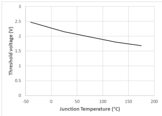
**Figure 9:** Threshold vs temp ( $I_{DS}=20\text{mA}$ ;
