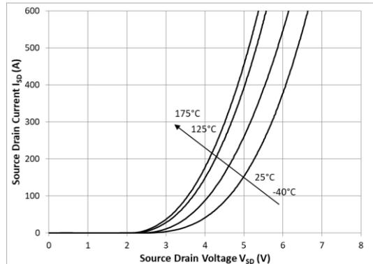
**Figure 6:** 3rd quadrant characteristics ( $V_{GS}=-3V$ ,  $t_p < 200\mu s$ )<sup>11</sup>
