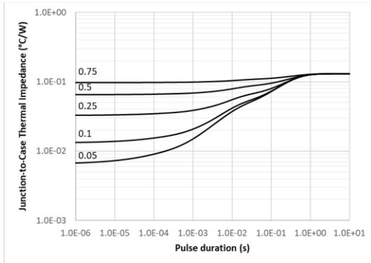
**Figure 15:** MOSFET Junction to Case Thermal Impedance
