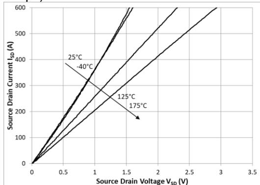
**Figure 5:** 3rd quadrant characteristics ( $V_{GS}=15V$ ,  $t_p < 200\mu s$ )<sup>11</sup>
