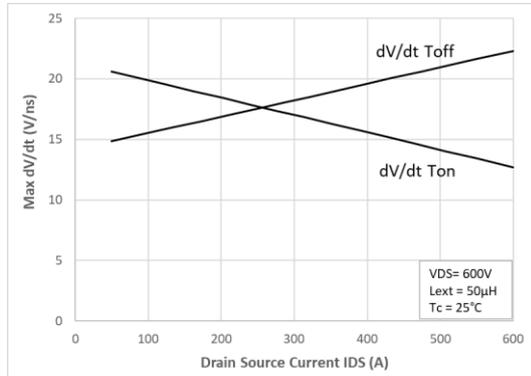
**Figure 12 :** Max dV/dt vs Drain current
