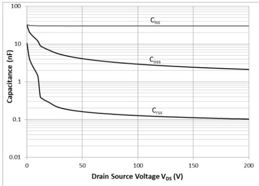
**Figure 7:** Typical capacitances vs  $V_{DS}$
