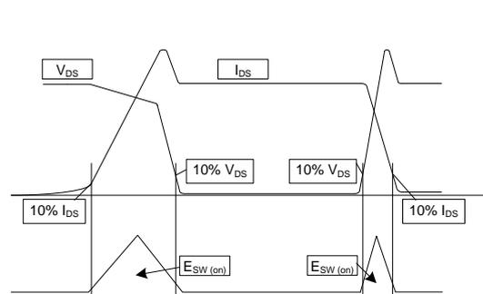
**Figure 14 :** Switching energy computation
