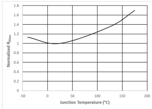
**Figure 3:** Normalized on-state drain source resistance ( $I_{DS}=300A$ ,  $V_{GS}=15V$ ,  $t_p < 200\mu s$ )<sup>11</sup>
