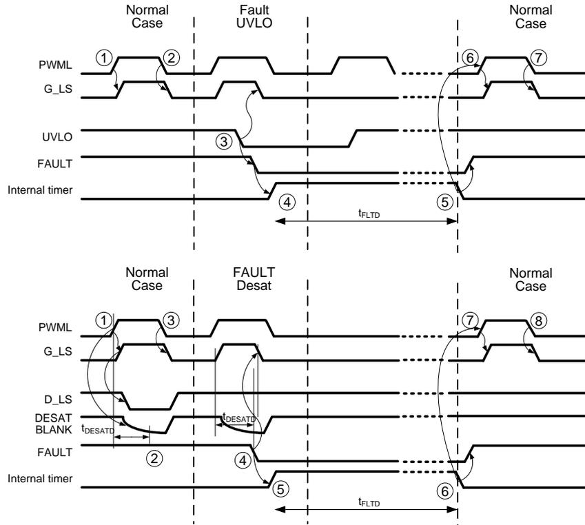
**Figure 2: Timing diagram CMT-TIT8243/8244 low-side driver behaviour**
