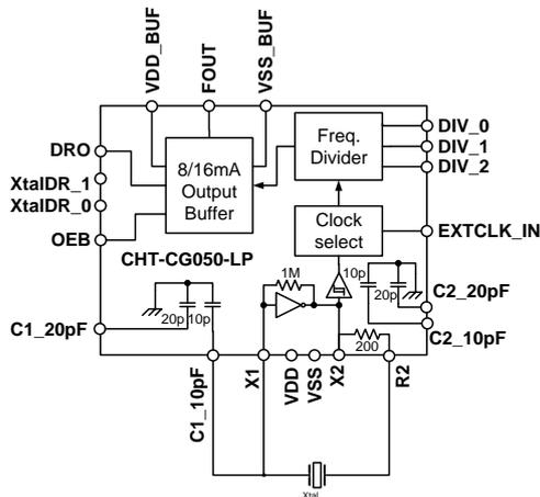
**Figure 9.** Minimal configuration.
