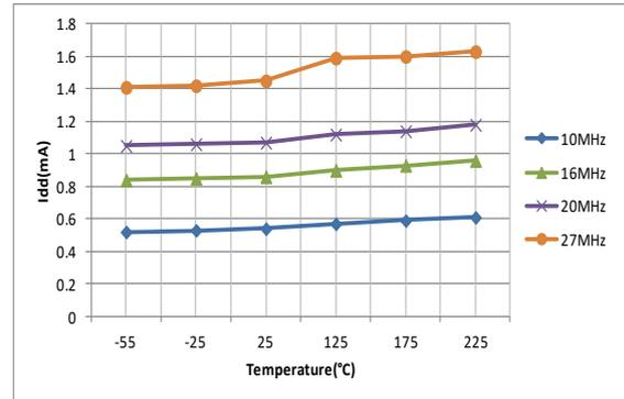
**Figure 2:** Current consumption ( $V_{DD} = 3.3V$ , OEB = LOW,  $C_L = 0pF$ , XTALDR\_0=1, XTALDR\_1=0)
