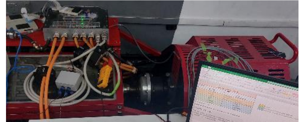
Inverter efficiency > 99% @ 700V/275Arms/10kHz
