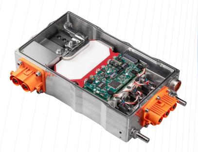
The high power density, easily configurable On-Board SiC Inverter Reference Design, has been developed to be one step closer to production-ready. This reference design is targeted for in-vehicle and field testing, further accelerating time-to-market and reducing engineering required to achieve a functional electric drive train.
