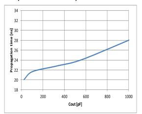
Figure 5: Propagation delay vs output capacitance (overdrive= 20mV, T<sub>a</sub> =25°C)
