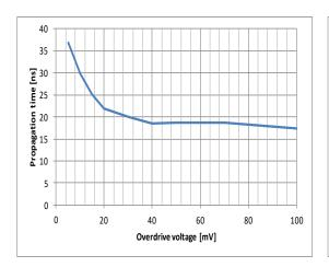
Figure 1: Propagation delay vs overdrive voltage  $(T_a = 25^{\circ}C)$
