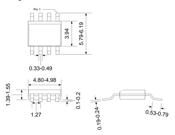
PSOIC8 physical dimensions (mm +/- 10%)
