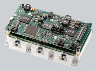
The SiC Inverter Control Module (ICM) is built based on CISSOIDs CXT-PLA3S series Intelligent Power Modules and HADES2 gate driver chipset, adding the new control board to the stack.
