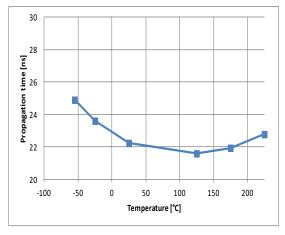
Figure 3: Propagation delay vs temperature (overdrive= 20mV)
