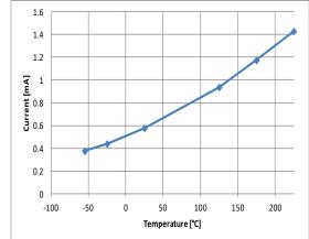
Figure 8: Static current vs temperature
