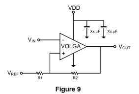
By increasing the hysteresis, sensitivity to noise (external noise, switching noise) is decreased.
