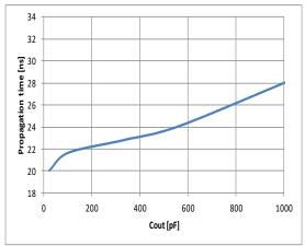
Figure 6: Propagation delay vs output capacitance (overdrive= 100mV,  $T_a = 25$ °C)
