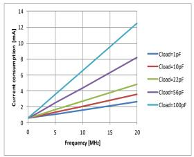
Figure 2: Current consumption vs frequency and load ( $T_a = 25^{\circ}C$ )
