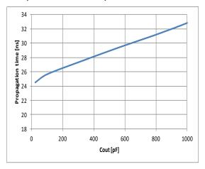
Figure 5: Propagation delay vs output capacitance (overdrive= 20 mV, T<sub>a</sub> = $25^{\circ}$ C)
