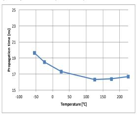
Figure 4: Propagation delay vs temperature (overdrive= 100mV)
