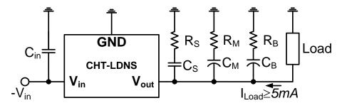
A minimum load current of 5mA is required. Bellow this value, a small oscillation of few tens of mV can occurs at the regulator output.
