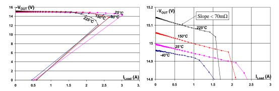
Figure 1: -Vout vs.ILoad (@2V dropout)
