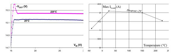
Figure 5: -Vout vs. -Vin over T° (Iload=60mA)
