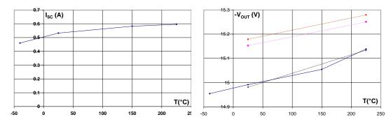
Figure 3:Short-circuit current vs. T°
