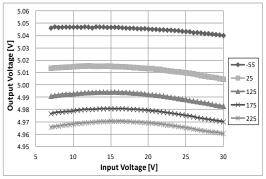
Figure 8: Voltage regulator line regulation ((VDD-VSS) from 7V to 30V; lout=2.5mA)
