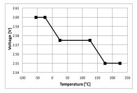
Figure 12. UVLO threshold
