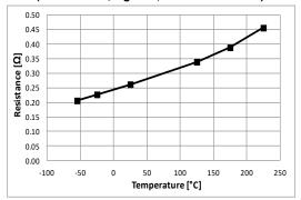
Figure 6: High-side output resistance
