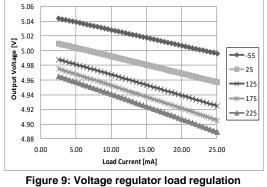
Figure 9: Voltage regulator load regulation (lout from 2.5mA to 25mA; (VDD-VSS)= 25V)
