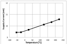
Figure 19. Quiescent current I<sub>q</sub>(VDD\_DESAT) (any PWM frequency; fault or no fault state; [VDD\_DESAT-VSS]=25V)
