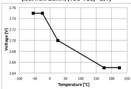
Figure 11. DESAT threshold
