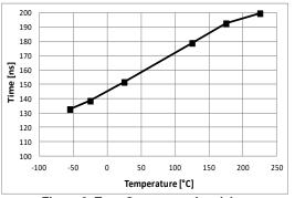
Figure 2: Turn-On propagation delay (from 50% RXP/PWM to OUT 10%; Cload = 1nF; TRX\_MODE=0)
