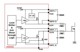
Figure 27 Output stage architecture
