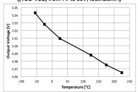
Figure 10: Voltage regulator (lout from 2.5mA; (VDD-VSS)= 25V)
