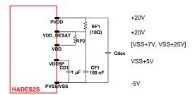
Figure 31. Power supplies configuration (MOSFET case)
