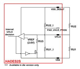
Figure 23: UVLO detection function
