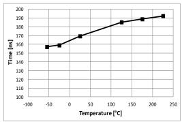
Figure 1: Turn-Off propagation delay (from 50% RXP/PWM to OUT 90%; Cload = 1nF;
