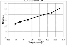
Figure 4: Turn-On rise time (Cload = 1nF; Rg= 5Ω; PVDD-PVSS=25V)
