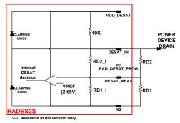
Figure 25: DESAT detection function
