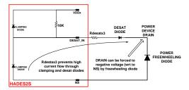
Figure 24: DESAT clamping circuit
