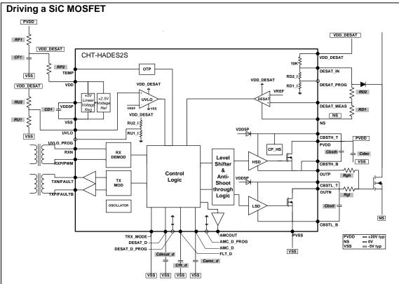
Figure 32: Typical application schematic (SiC MOSFET power device)
