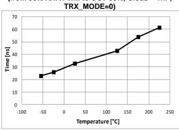
Figure 3: Turn-Off fall time (Cload = 1nF; Rg=  $5\Omega$ ; PVDD-PVSS=25V)
