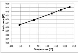
Figure 5: Low-side output resistance
