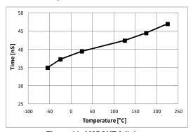
Figure 14. AMCOUT fall time (Cload on AMCOUT: 0.5 nF)
