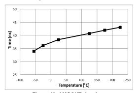
Figure 13. AMCOUT rise time (Cload on AMCOUT: 0.5 nF)
