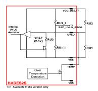
Figure 30: Fault generation by over temperature event
