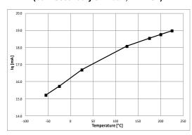
Figure 31. Average current VIN (no fault, DINx=20kHz 50% DC; VIN=15V)
