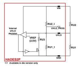
Figure 33: UVLO detection function
