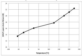
Figure 11: DOUT open drain Ron (VIN=15V)
