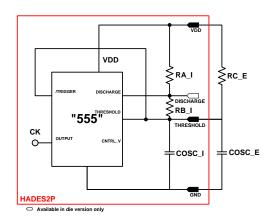
Figure 36: Oscillator with external components (for packaged version)
