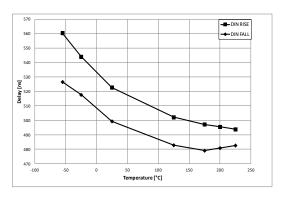
Figure 8: DIN->TX Propagation Delay (modulated interface; spike filter on)
