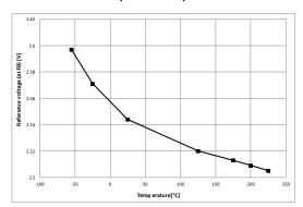
Figure 5: Voltage reference @ FB pin (including OPA offset)
