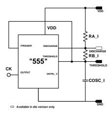
Figure 35: Internal oscillator scheme (for die version)
