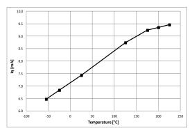
Figure 30. Average current VIN (no fault, DINx=0; VIN=15V)
