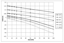
Figure 4: Voltage regulator load regulation (Vin=15V)
