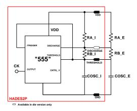
Figure 37: Oscillator with external components (die version)
