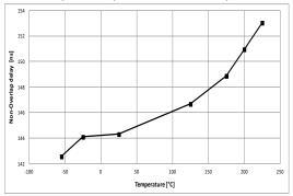
Figure 12: Non-Overlap delay (no external capacitor)
