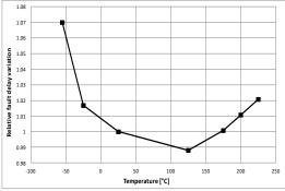
Figure 13. Fault timer tFLT\_D (CFLT\_D=20nF).
