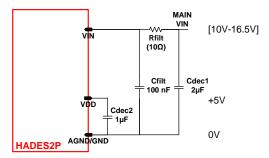
Figure 41. Power supplies configuration and decoupling
