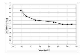
Figure 1. UVLO threshold
