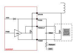
Figure 40. DC-DC output stage
