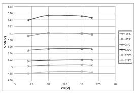
Figure 3: Voltage regulator line regulation (lout =3 mA)
