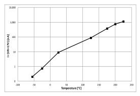
Figure 21: AUX diode Vf (If=1mA)
