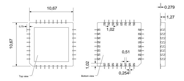
CQFP32 physical dimensions in mm (tolerance : +/- 0.2 mm)
