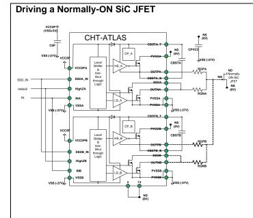
The normally-ON SiC JFET is turned off once the gate-source voltage drops below the negative pinch-off voltage of the JFET. At zero gate-source voltage, the device is fully ON. For proper gate drive, CHT-ATLAS has its positive supply pins (PVCCA/B) tied to the source of the JFET (NS). Its negative supply pins (PVSSA/B) are connected to a negative voltage power supply with respect to NS.
