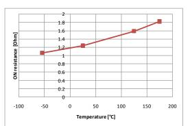
Figure 6: High-state output resistance vs. Temperature
