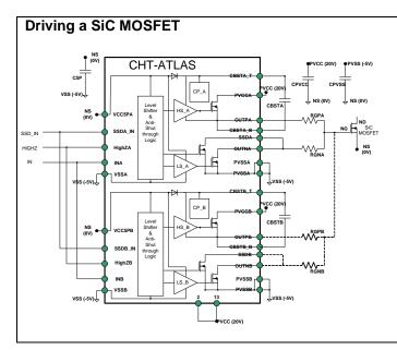
Driving a SiC MOSFET requires a gate driver capable of a large gate voltage swing and fast gate voltage transitions.
