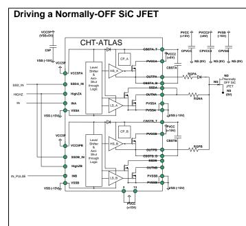
Unlike the normally-on JFET, the gatesource junction of the normally-off SiC JFET is forward biased in the device conduction state. In addition to the dynamic current for charging/discharging the total gate capacitance, some steadystate current has to be provided to maintain conduction after the device has been switched on.
