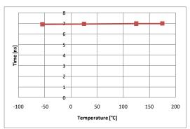
Figure 4: Turn-High Rise Time vs. Temperature
