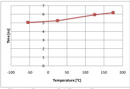
Figure 3: Turn-Low Fall Time vs. Temperature
