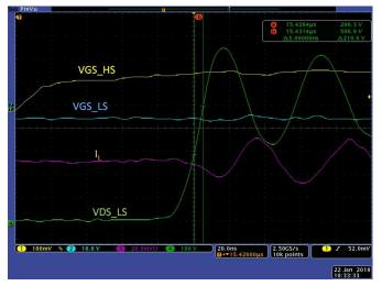
Figure 5: dV/dt>40KV/µs at turn-on with CMT-TIT8243 gate driver and CAS300M12BM2 module [5]
