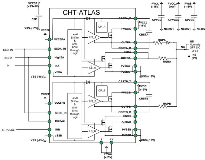
Unlike the normally-on JFET, the gate-source junction of the normally-off SiC JFET is forward biased in the device conduction state. In addition to the dynamic current for charging/discharging the total gate capacitance, some steady-state current has to be provided to maintain conduction after the device has been switched on.
