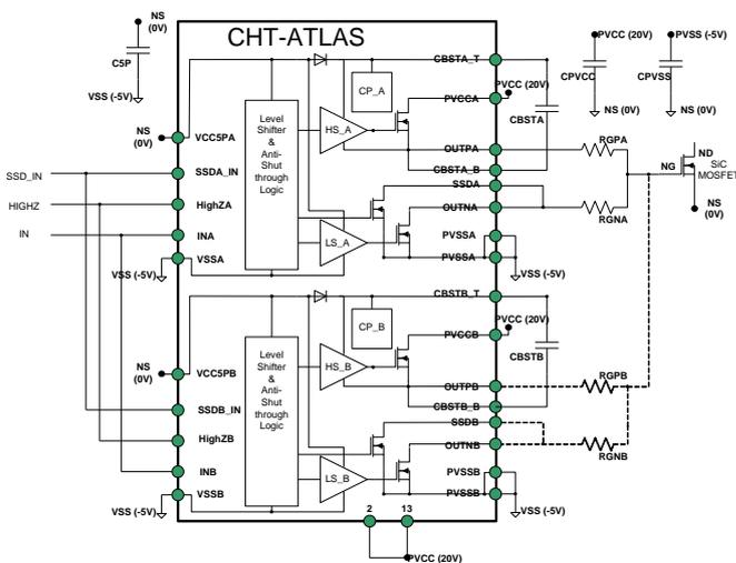
Driving a SiC MOSFET requires a gate driver capable of a large gate voltage swing and fast gate voltage transitions.
