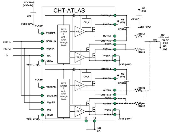
The normally-ON SiC JFET is turned off once the gate-source voltage drops below the negative pinch-off voltage of the JFET. At zero gate-source voltage, the device is fully ON. For proper gate drive, CHT-ATLAS has its positive supply pins (PVCCA/B) tied to the source of the JFET (NS). Its negative supply pins (PVSSA/B) are connected to a negative voltage power supply with respect to NS.
